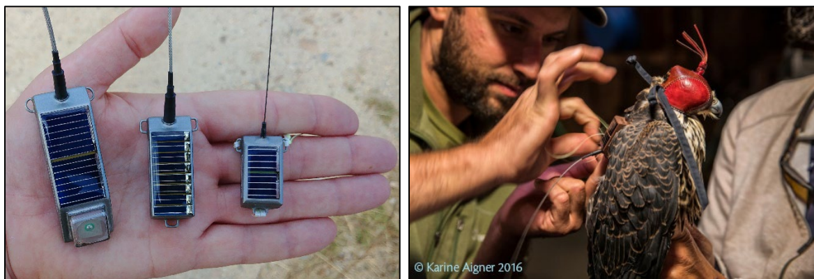
Figure 4. Left: Example of 22g solar GPS PTT unit, 12g solar PTT and 5g solar PTT unit used to track movements of Peregrine Falcons, Merlins and Northern Harriers. Right: A hooded Peregrine Falcon being fitted with a transmitter (right).
